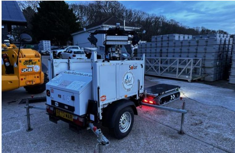
The SMC TL55 Solar meets the demand for a sustainable, environmentally friendly and low maintenance lighting tower. Reliable, robust and offering instant light from four 60W LED lamps, the SMC TL55 Solar does not compromise on power or quality. With both battery and mains supply provision, it offers flexible options for all applications on site with an indefinite run time.
