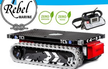
The TC1 carrier is the solution for transport of long, heavy materials, equipment and pontoons at a project site. The carrier is compact and just 80 cm wide, and items can be placed on it in the length or width. The radio remote controlled carrier is perfect for transporting material, such as steel beams, through small access doors and less easily accessible areas. No more heavy lifting for your personnel. Ergonomic, efficient and safe!
